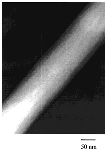
Figure 2. TEM image (negative) of a 150 nm diameter poly-(ferrocenyldimethylsilane) nanofiber.
